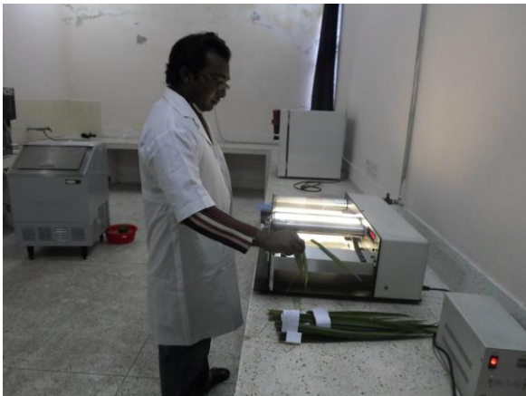
Figure 1: Measurement of leaf area in BAU central lab by LI-3100 Area Meter Instrument.
